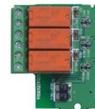
■ EME-R3AA Relay card (3 form A/ NO contacts)
